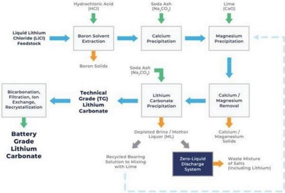
The chemical conversion process of lithium chloride to BGLC is shown above
