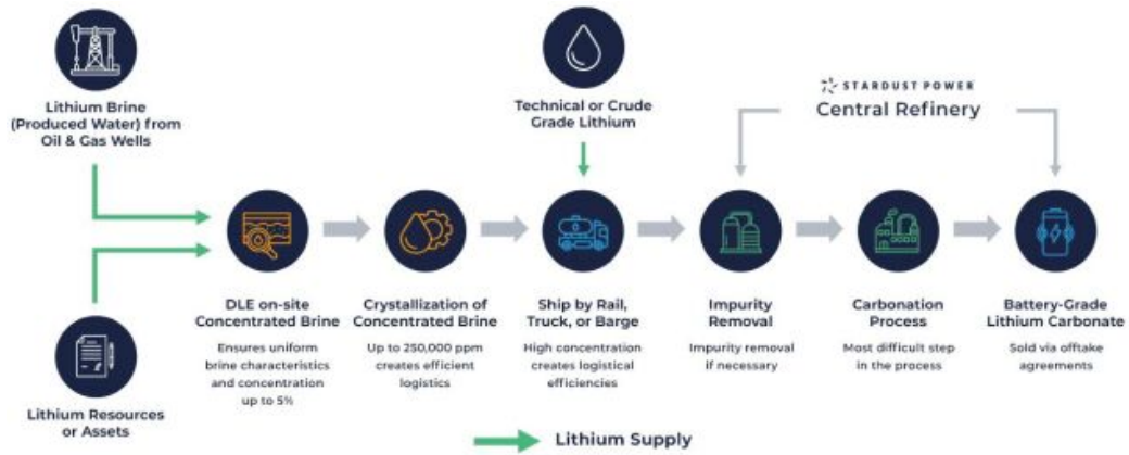
The chart above shows the ability of a central refinery to process multiple inputs or multiple sources of supply, which enables Stardust Power to have a diversified supply chain.
